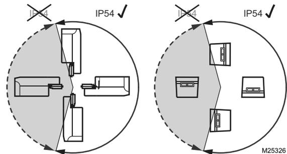
Fig. 8. Mounting for IP54.
